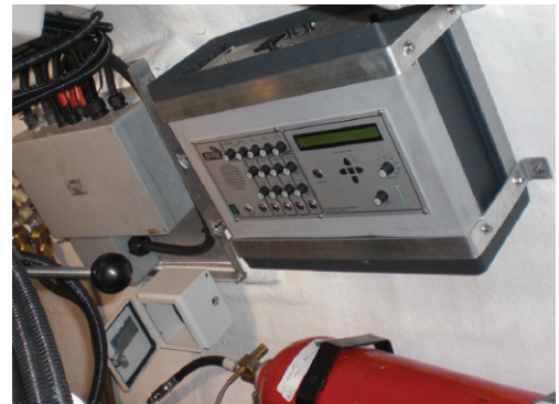
HeliCom™ Unscrambler inside hyperbaric lifeboat.
